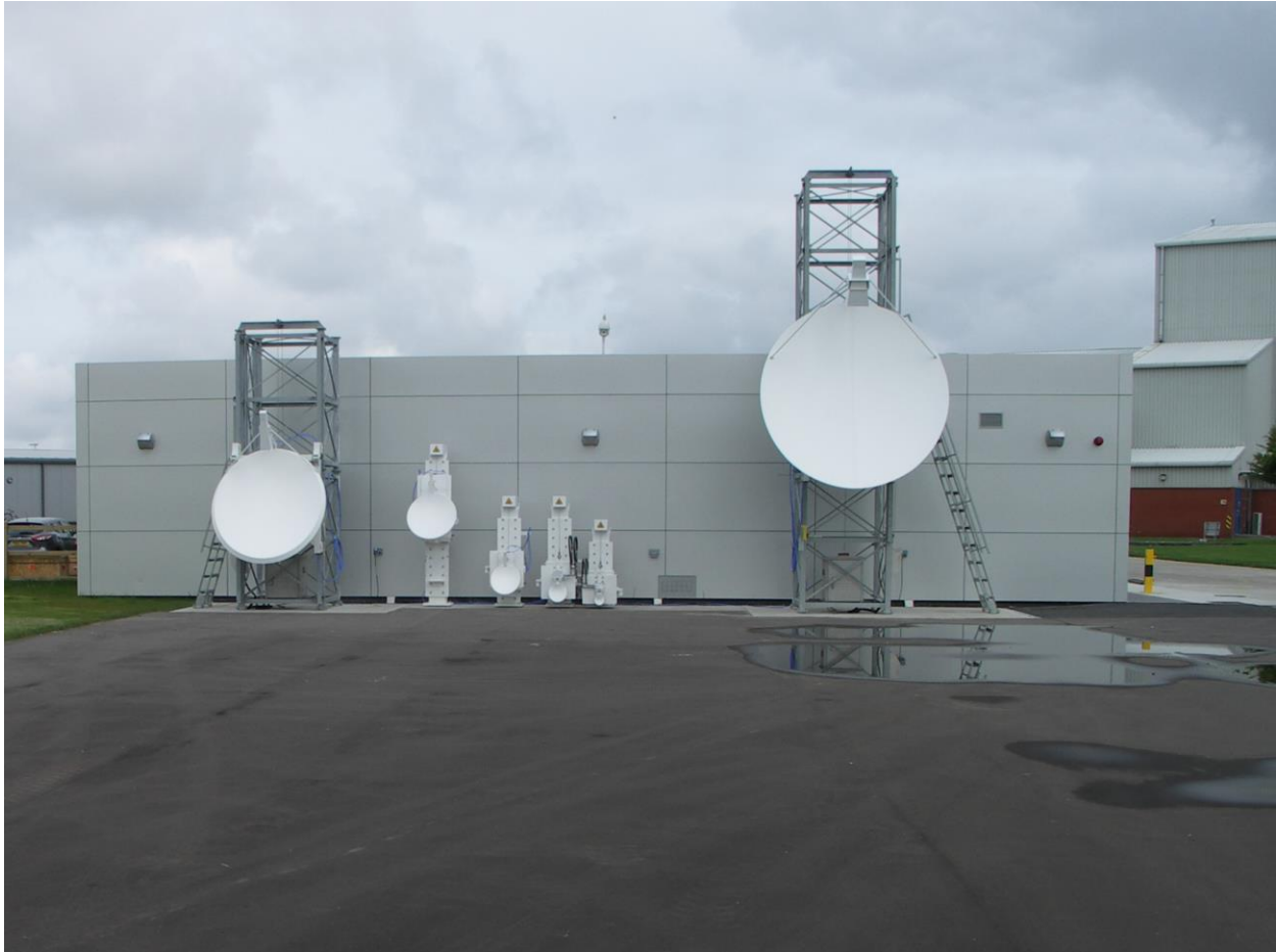
0.6 – 18 GHz, Dual Linear Polarization, RCS Range Antennas w/ Elevators
