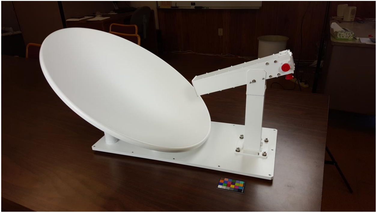
8-18 GHz, Dual Linear Polarization Offset
